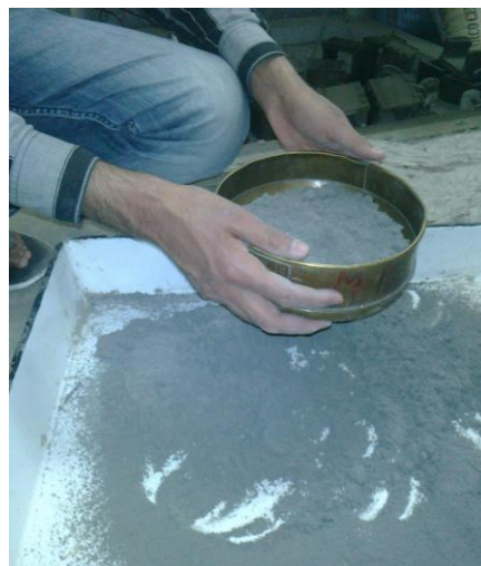
Fig. 2.7 Mixing of fly-ash with cement.
