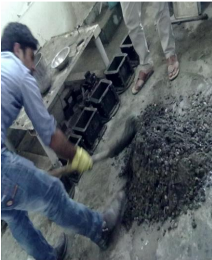
Fig.2.8 Mixing of concrete.
