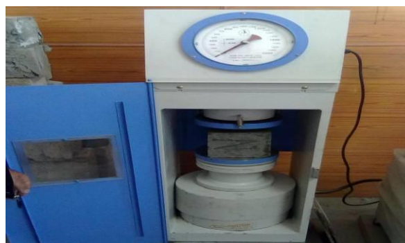
Fig. 2.2 Compressive strength test in a CTM
