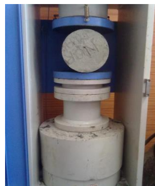
Fig. 2.5 Splitting tensile strength test in a CTM.
