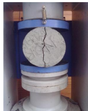
Fig. 2.6 Formation of crack along the diameter of cylinder.
