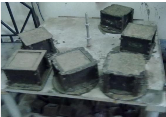
Fig. 2.9 Vibration of concrete cubes being done on a table vibrator.
