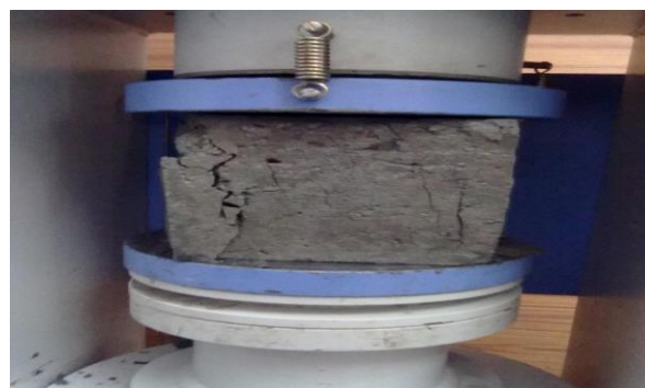
Fig. 2.3 Formation of cracks in Compressive strength test.
