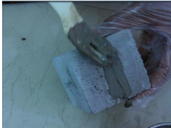
Fig. 4 – Inserting paste of Bacillus Sphaericus mixed with Fly ash in cracked portion
