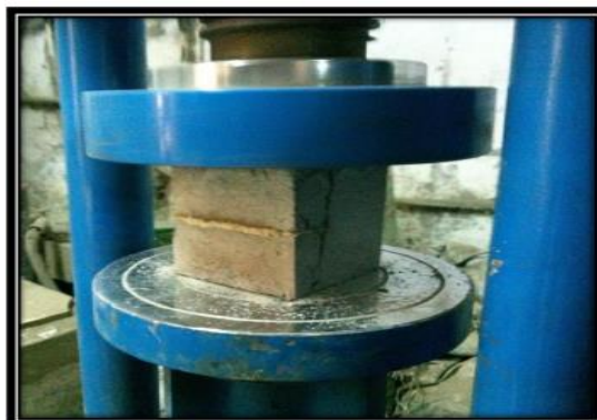
Fig 2 compression test setup
