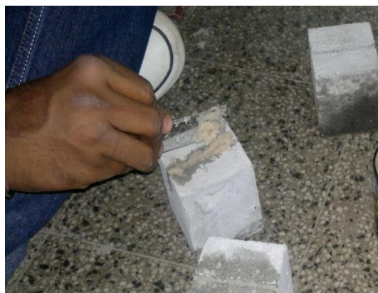
Fig. 4 – Inserting paste of Bacillus Pasteruii mixed with Ennore sand in cracked portion
