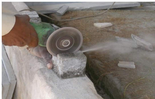
Fig. 3 creating artificial crack by marble cutter
