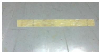
Fig.1 First sample with [0_G, 90_{BM}, 0_{BN}, 0_G] orientation
