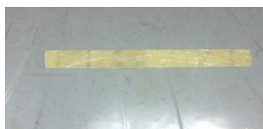
Fig.2 Second sample with [0_G, 90_{BM}, 0_{BN}, 0_G] orientation
