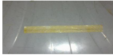
Fig.4 Fourth sample with [0 G , 0 BM , +45 BN , 0 G ] orientation
