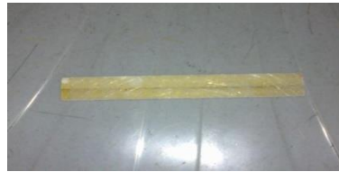
Fig.3 Third sample with [0 G , 0 BM , +45 BN , 0 G ] orientation
