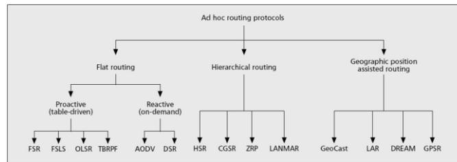
Figure 1 Classification of Routing Protocols
