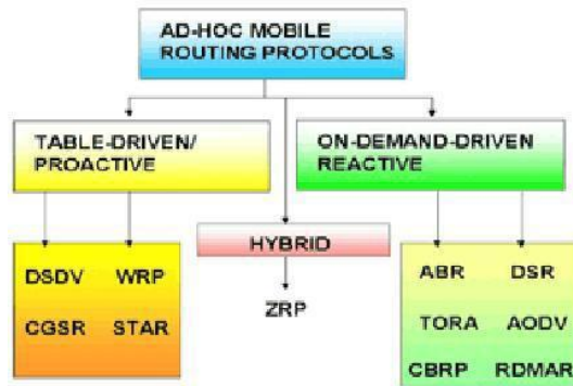
Fig 1 Classification of MANET routing Protocol
