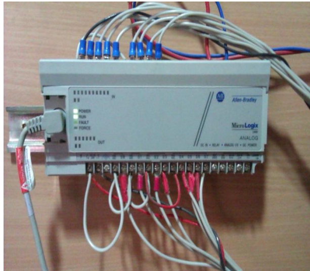
Figure 3.8 Allen Bradley Micrologix 1000
