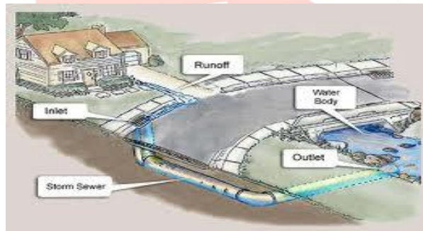
Fig 1 Typical Stormwater Drainage System
