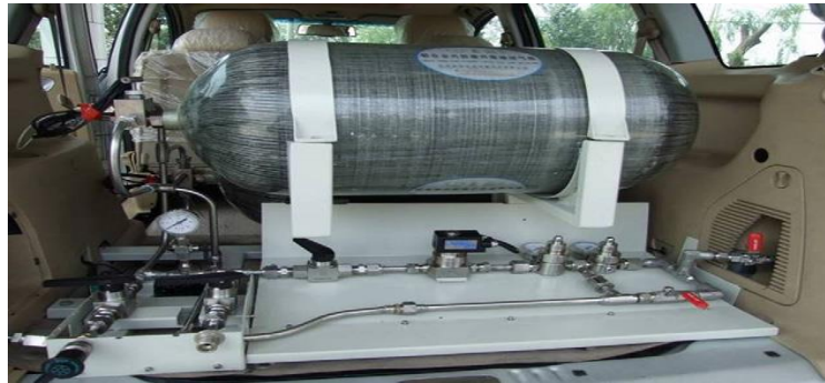
Fig. 1. Lightweight composite high-pressure hydrogen storage vessel used in the hydrogen fuel-cell vehicle.
