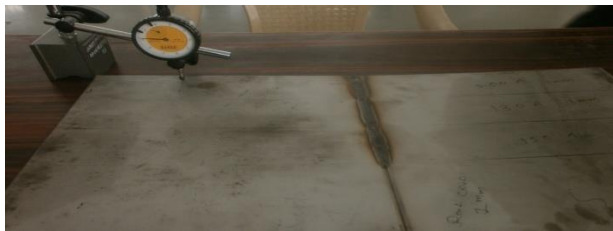
Figure 3. Measuring Distortion on welded part
