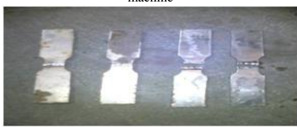
Figure 7. Tensile sample after testing
