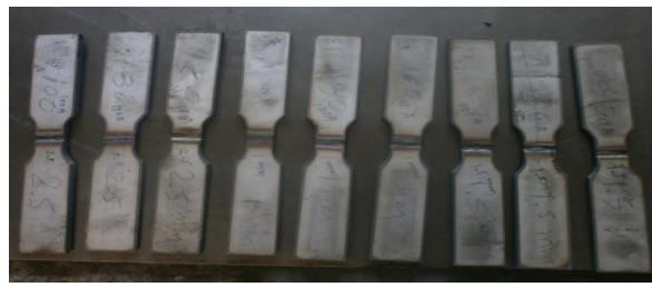
Figure 5. Tensile sample before testing
