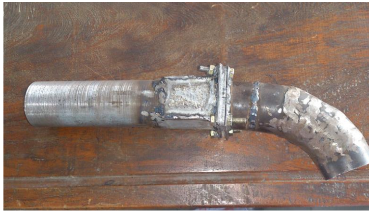
Figure 3.1- Side view of Resonance chamber
