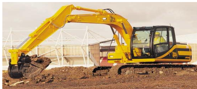
Fig. 1 JCB JS 130 (Tracked Excavator)
