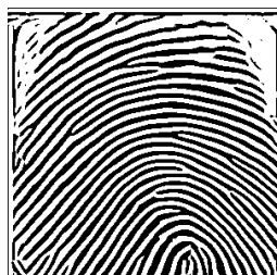
Figure.6 Image after the Gabor filter and Binarization
