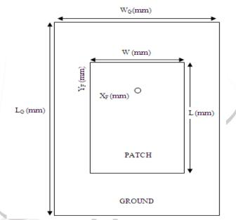
Fig.2. Schematic of the rectangular patch antenna
