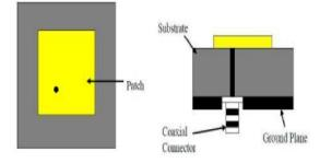
Fig.1. Co-ax fed patch antenna
