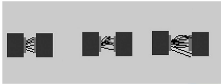
Figure 5c: Unwanted SWCNTs etched by O 2 plasma.
