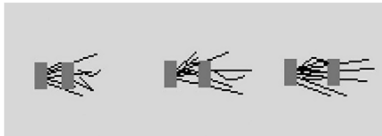
Figure 5b: Pd deposited for source and drain contact.
