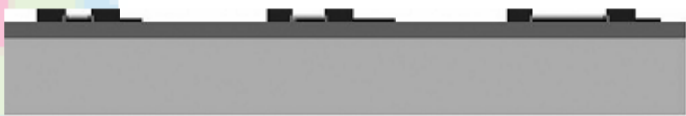
Figure 4i: Au deposited on source and drain contacts for probing purpose.
