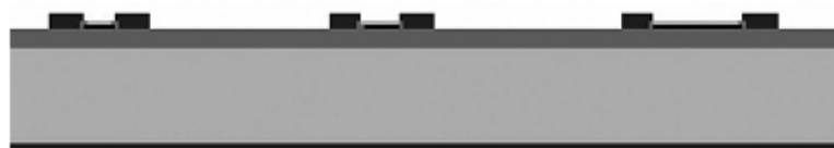
Figure 4l: Au deposition as gate contact at back side of the substrate.
