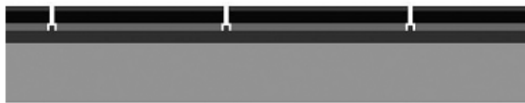
Figure 4d: Deposition of Pd for SWCNT growth.
