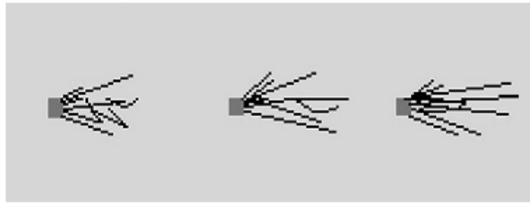
Figure 5a: SWCNTs grown by CVD technique.
