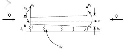
Fig.5 Beam on elastic foundation
