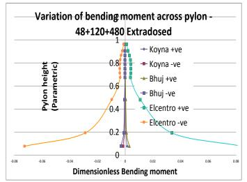
Fig.11 Variation of bending moment across pylon height for 48+120+48m span (Non-dimentionalized)
