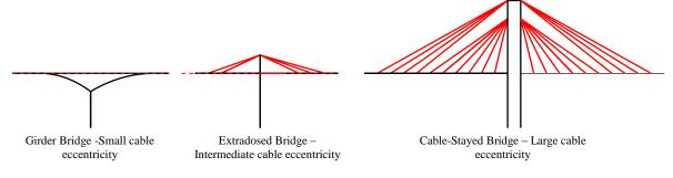
Fig. 1 Figure showing Cable arrangements in Girder Bridge, Extradosed Bridge and Cable stayed bridge Some features of Extradosed bridge as given below;
