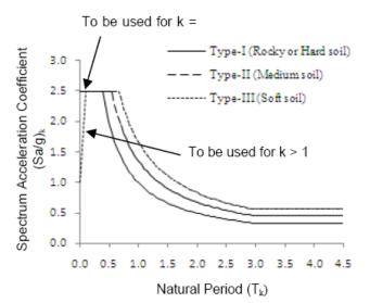
Fig. 3 Acceleration response for 5% damping used for response spectrum method
