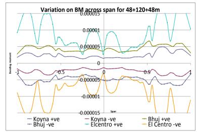
Fig.8 Variation of bending moment across span for 48+120+48m span (Non-dimentionalized)
