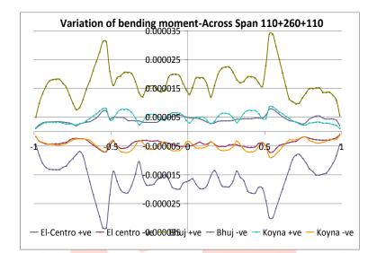
Fig.6 Variation of bending moment across span for 110+260+110m span (Non-dimentionalized)
