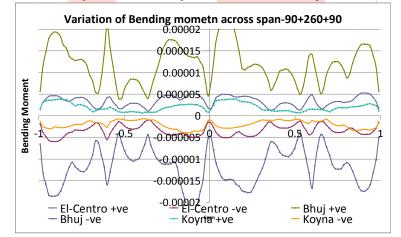
Fig.7 Variation of bending moment across span for 90+200+90m span (Non-dimentionalized)
