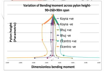
Fig.10 Variation of bending moment across pylon height for 90+200+90m span (Non-dimentionalized)
