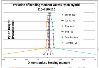
Fig.9 Variation of bending moment across pylon height for 110+260+110m span (Non-dimentionalized)
