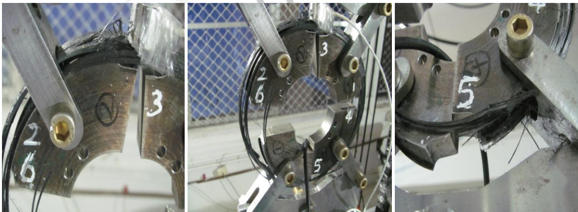
Fig. 6 Failure of specimen
