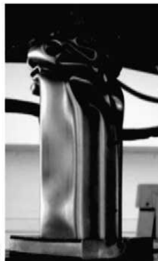
Fig. 7 Stable crushing ensured by cutting beams corners (a) beam without cut corners after crush test, (b) beam with cut corners after crush test [7]
