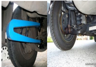
Fig 2 : Location of Coil Spring and composite spring at rear suspension
