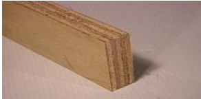
Plywood is a common composite material that many people encounter in their everyday lives
