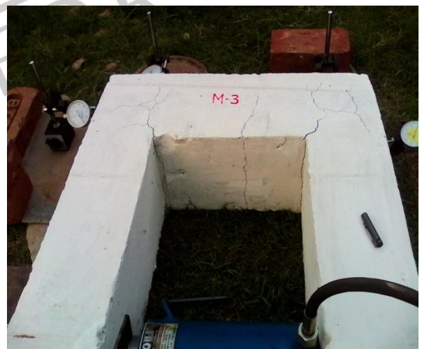
PLATE- 3.3 Process of retrofitting and cracks development after testing
