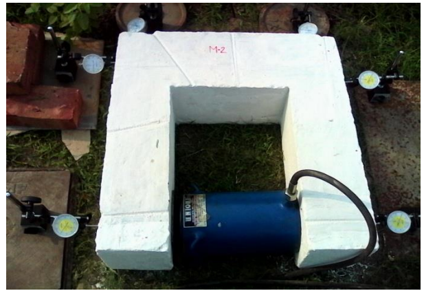
Plate – 3.2 Hydraulic jack installed on beam column joint
