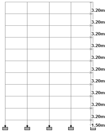
Figure 1 Elevation of the building
