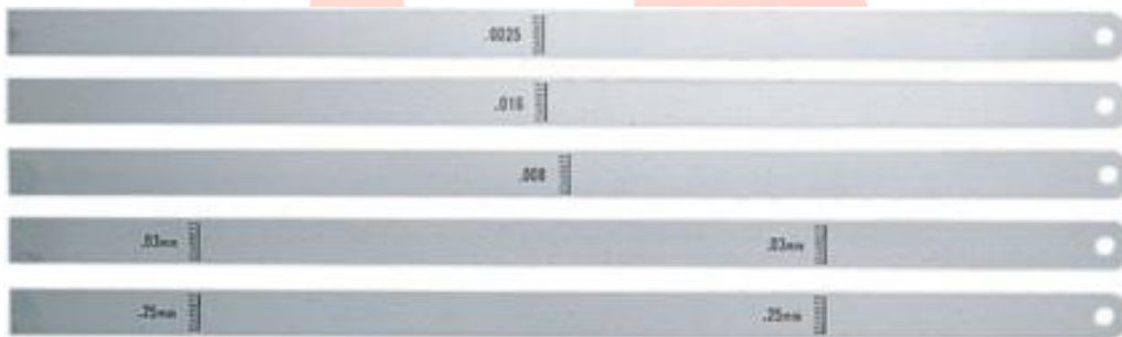
Figure 8.4 Shims used in tappet setting
