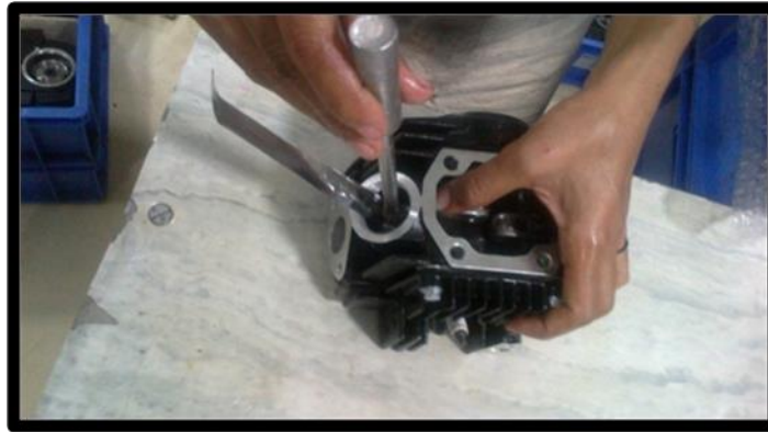
Figure 5.1 Tappet setting at sub assembly station
