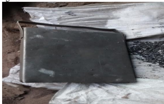
Figure-5: Plate type Magnetic Separator
