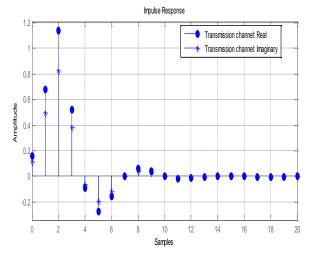
The received signal x[n] is generated by the transmitted signal s[n] filtered by the channel impulse response with additive noise v[n]. We shall assume a complex Gaussian noise signal for the additive  $n\setminus$
