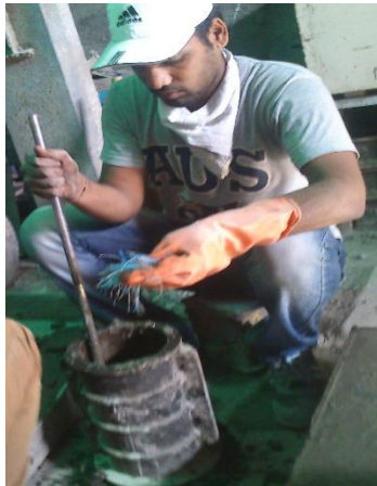
Fig 2: Casting of cylinder
