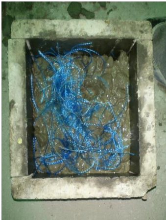
Fig 1: Casting of cube
