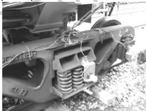
Fig. 31: Instrumented modified design bogie
