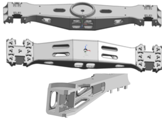
Fig. 14: Modified bolster solid model.
