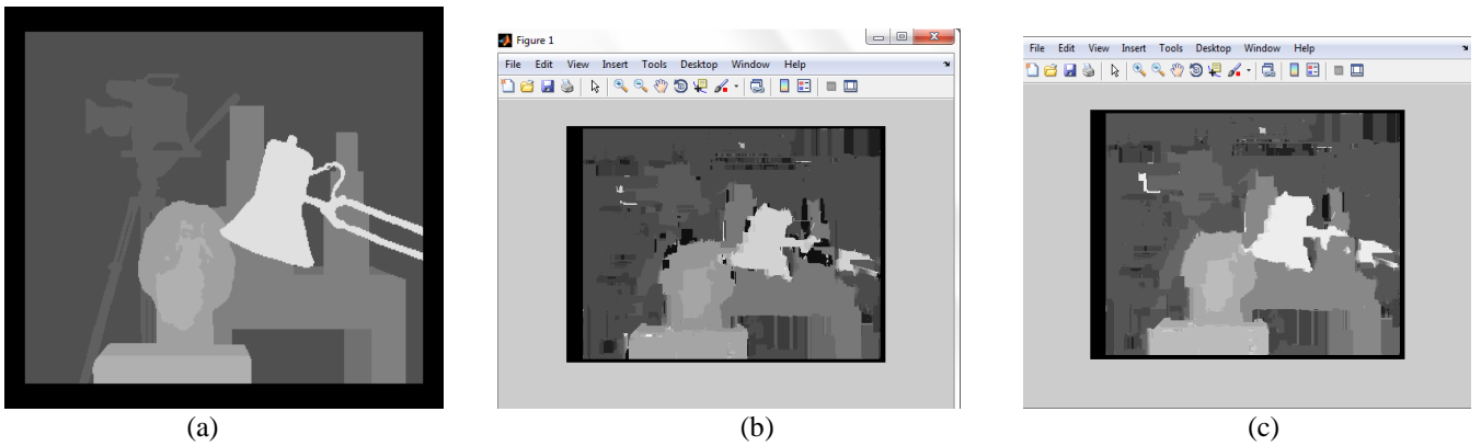
Figure 2 (a) tsukuba image pair ground truth map,(b) disparity map of existing method ,(c) disparity map of proposed method
