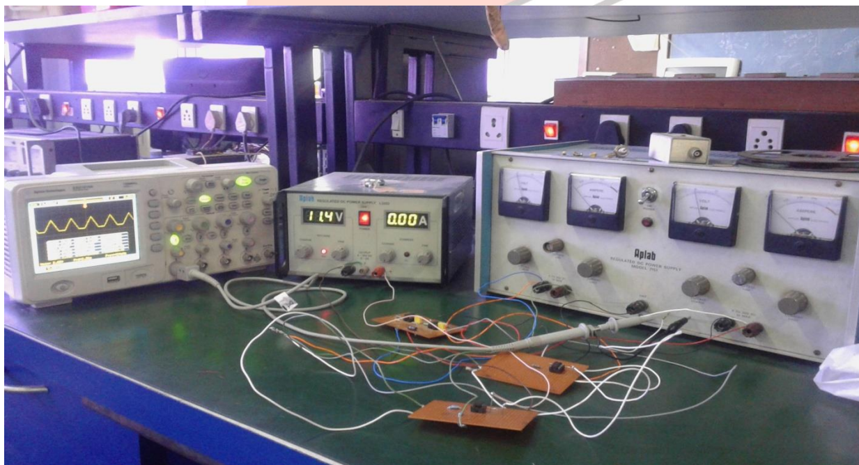
Figure 6 A assembly of hardware testing of differential amplifier
