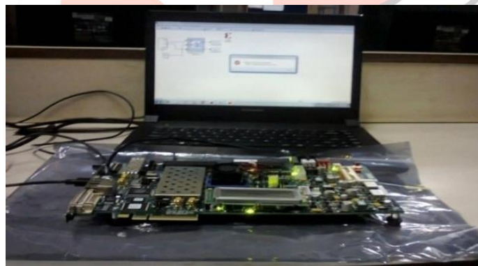
Figure 8 Setup for Co-hardware Simulation using ML605 Board.
