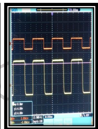
Fig.7(c) Driver Circuit Output at Duty Ratio is 60%
