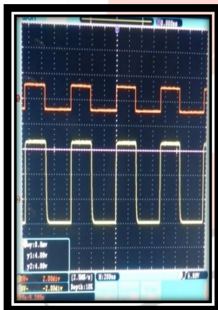
Fig.7(b) Driver Circuit Output at Duty Ratio is 40%
