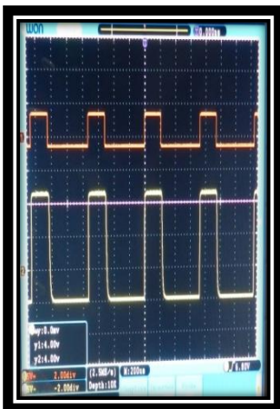
Fig.7(a) Driver Circuit Output at Duty Ratio is 30%
