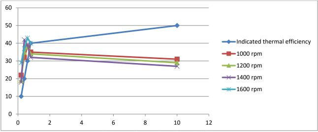
Equivalence ratio Vs Indicated thermal efficiency
