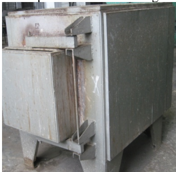
Fig.3: Electric muffle furnace
