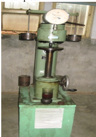
Fig. 9: Brinell Hardness Testing Machine
