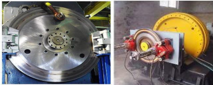
Fig-1: Disc brake with two calipers in Wind Turbines
