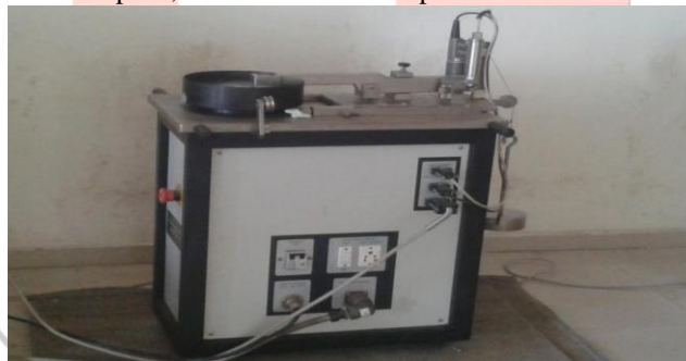
Fig. 4: pin on disc wear testing machine [27]
