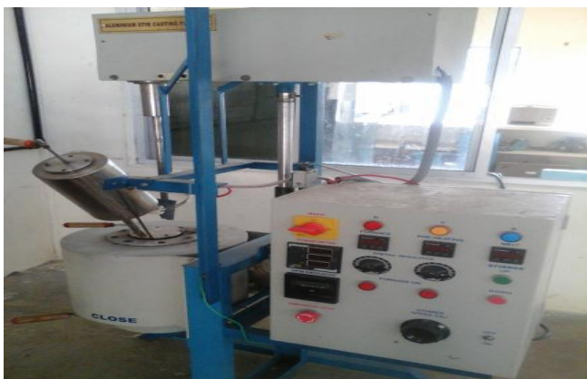
Fig. 2: stir casting machine set up
