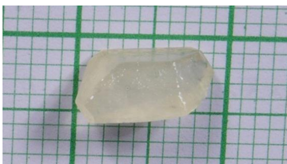
Figure 2 Photograph of as grown BGLM single crystal
