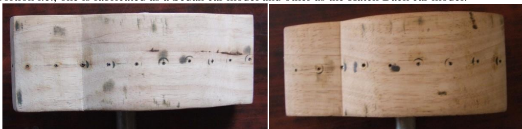
(a) (b) Fig. 4 Scaled wooden car models: (a) Sedan; (b) Hatch Back
