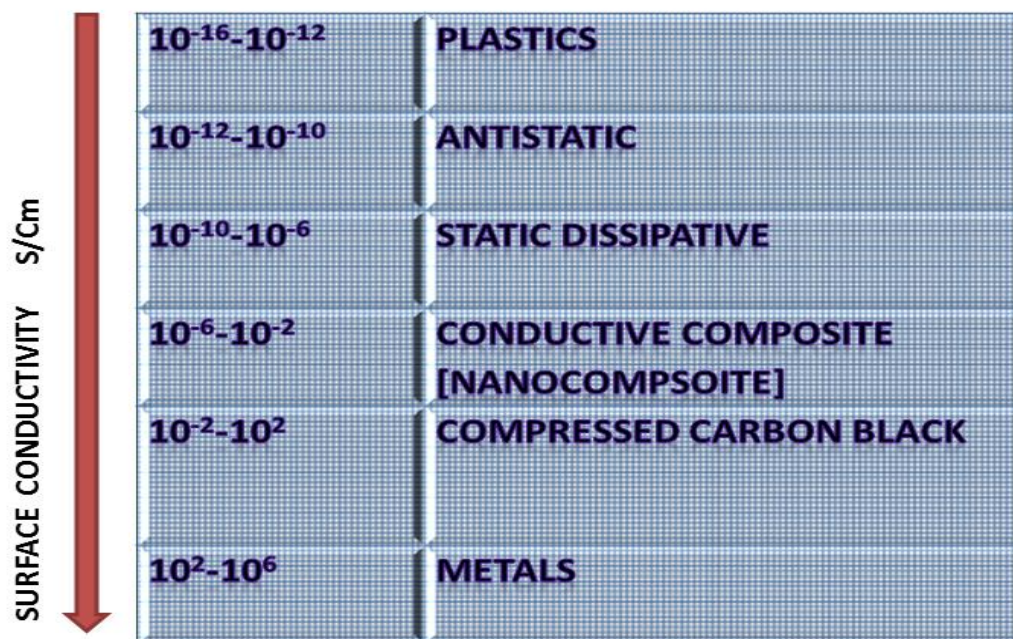
Figure 1: Applications of materials on the basis of conductivity range
