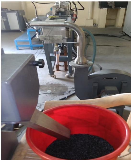
Figure 5: The running Twin Screw Extruder lab set up for master batch production
