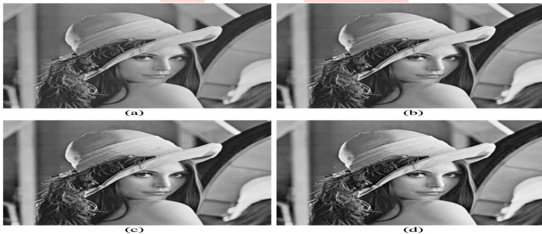
Fig. 4. The original and contrast-enhanced images of “Lena” by splitting 10, 15 and 20 pairs of histogram peaks in the proposed algorithm. (a) Original image of “Lena”. (b) 10 pairs: 0.185 bpp, 29.10 dB. (c) 15 pairs: 0.268 bpp, 25.97 dB. (d) 20 pairs: 0.345 bpp, 24.91 dB.
