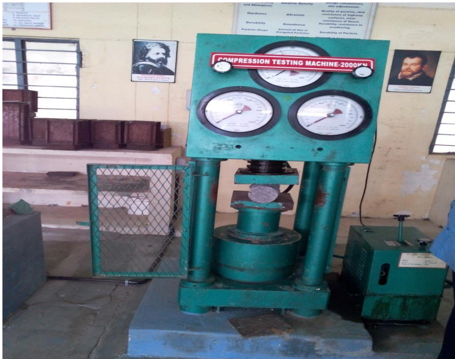
Fig4. Split tensile strength testing
