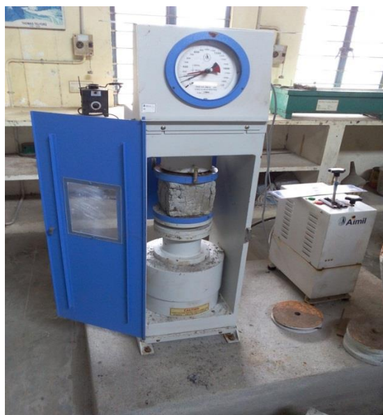
Fig.1 compressive strength testing
