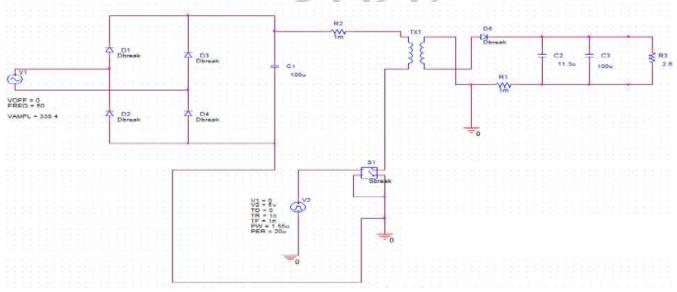
Figure 13: Simulated circuit of cell charger with voltage ripple less than 5%.
