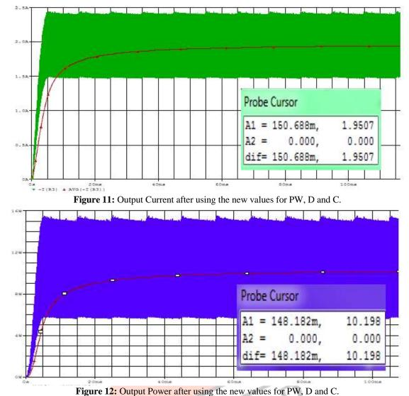
Figure 11 illustrates that the output current of the circuit is 1.95 A. The output value for power is 10.19 W as shown in figure 12.
