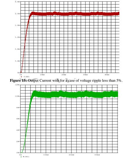
Figure 16: Output power with for a case of voltage ripple less than 5%.
