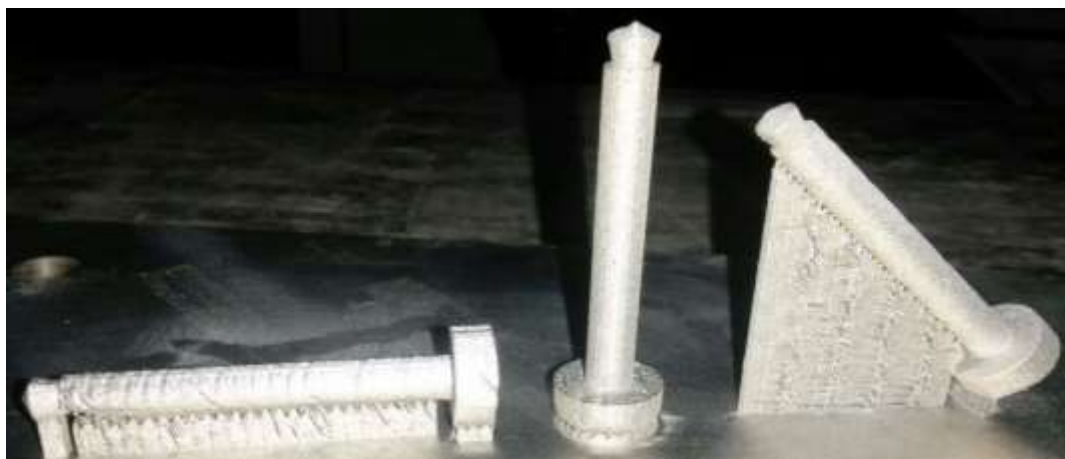
Figure 3.Part fabricated by SLS Process
