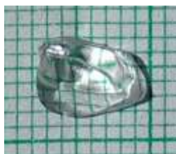
Fig.1 Photograph of the as grown single crystal of L-Isoleucine D-Alanine
