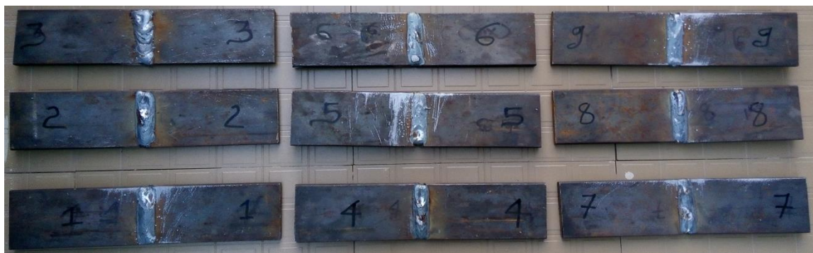
Fig.5. Work pieces after MIG Welding
