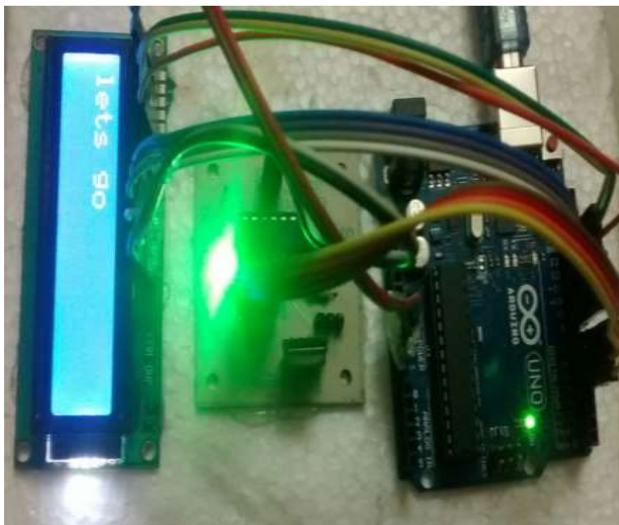
Figure 7: LCD display in the transmitter section to describe the status of movement of the robotic vehicle.
