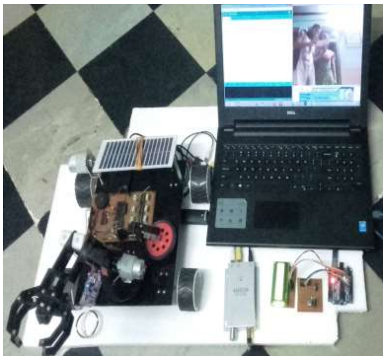
Figure 5: Transmission section through which inputs are given to robot by using ARDUINO IDE software
