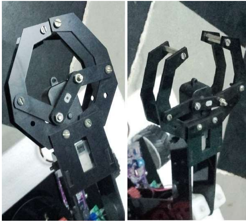
Figure 11: Robotic arm with its gripper close and open which is used to pick and place any object.
