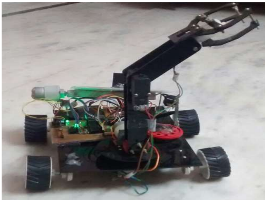
Figure 10: Robotic arm moving anti clockwise direction and also moves in clockwise about 270 degrees
