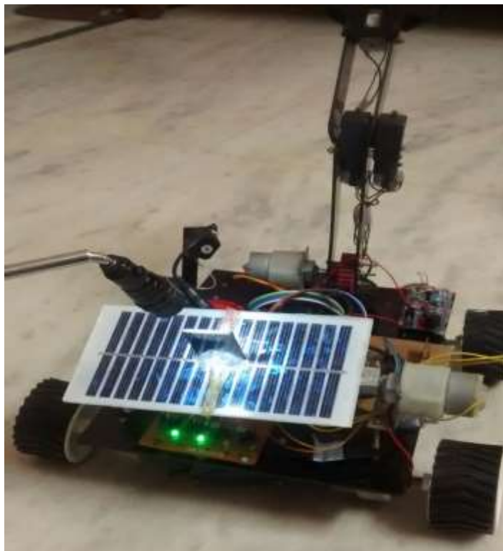
Figure 14: solar panel used in this project which is used to store solar energy with 9volts of voltage and 500mA of current.
