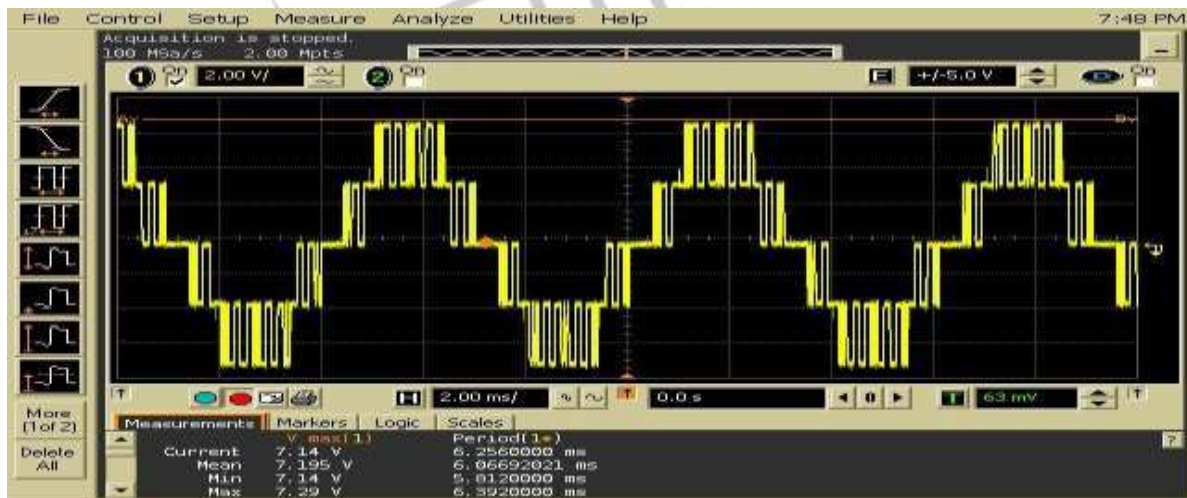
Fig 15: Output of SHMLI – Power Circuit
