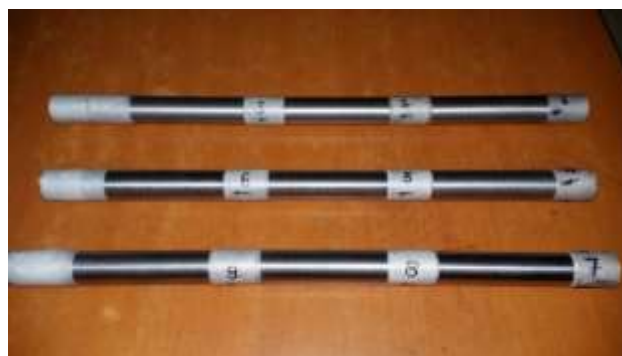
Fig. 1: Specimen photograph after machined
