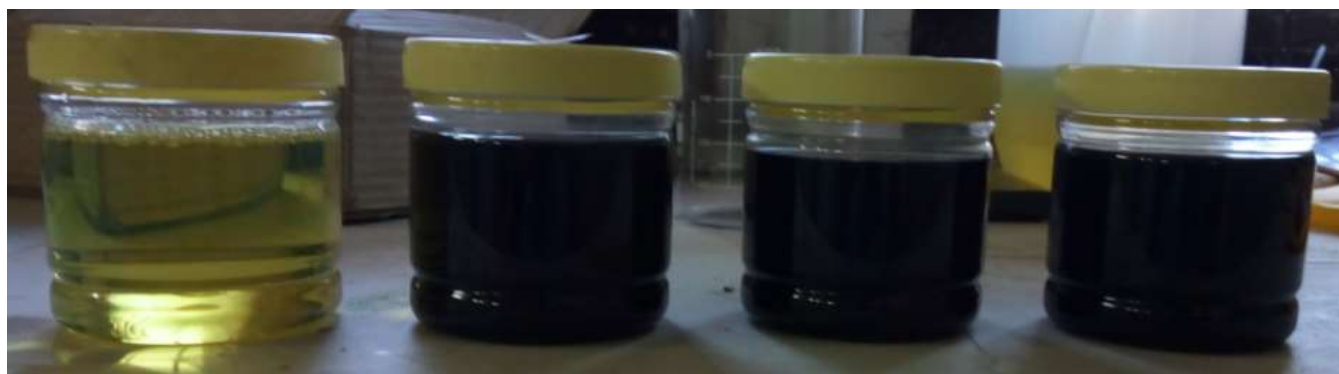
Fig 2 Photograph of diesel and its blends with MWCNT
