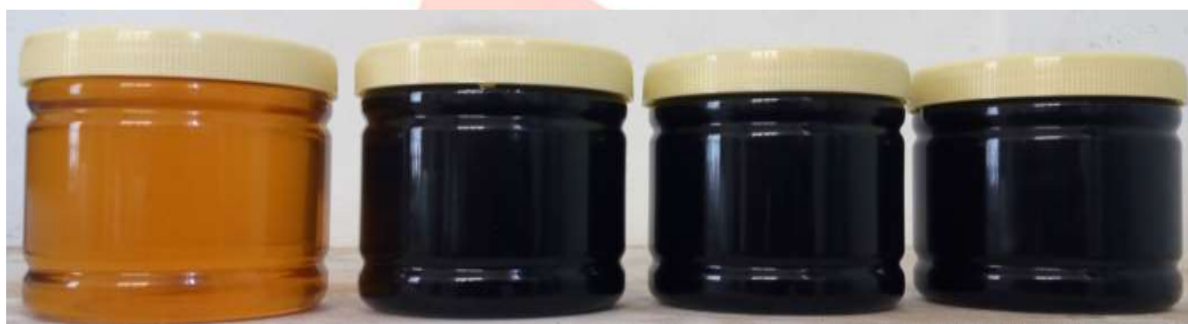
Fig 3 Photograph of karanja biodiesel and its blends with MWCNT
