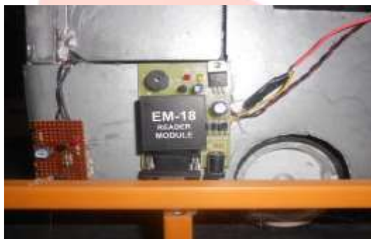
Figure: RFID reader and vibration sensor at the entrance of the bus
