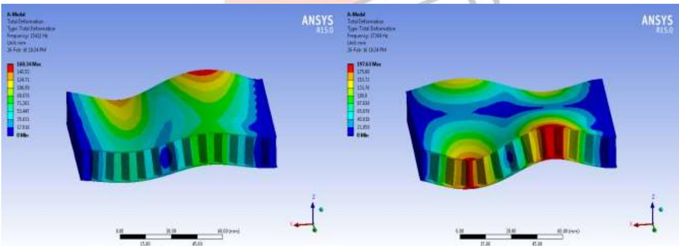
Fig 4.9 For mode 5 and 6 total deformation result of hexagonal core
