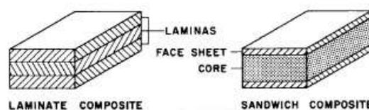
Fig 1.1 Laminate composite and sandwich composite
