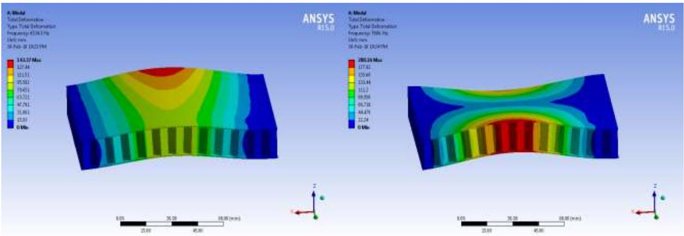
Fig 4.7 For mode 1 and 2 total deformation result of hexagonal core
