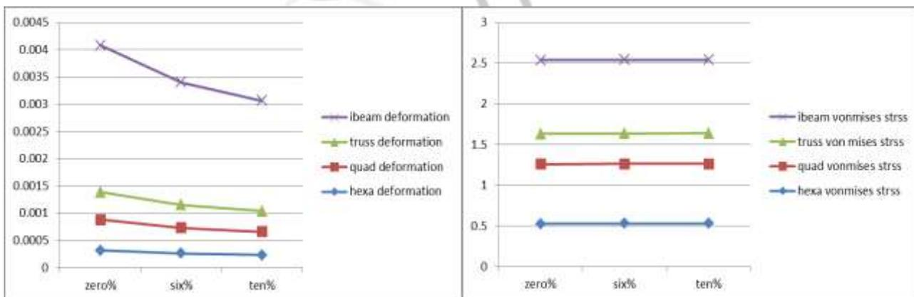
Graph 5.5 Overall dynamic deformation Graph 5.6 Overall dynamic vonmises stress
