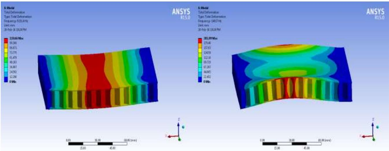
Fig 4.8 For mode 3 and 4 total deformation result of hexagonal core
