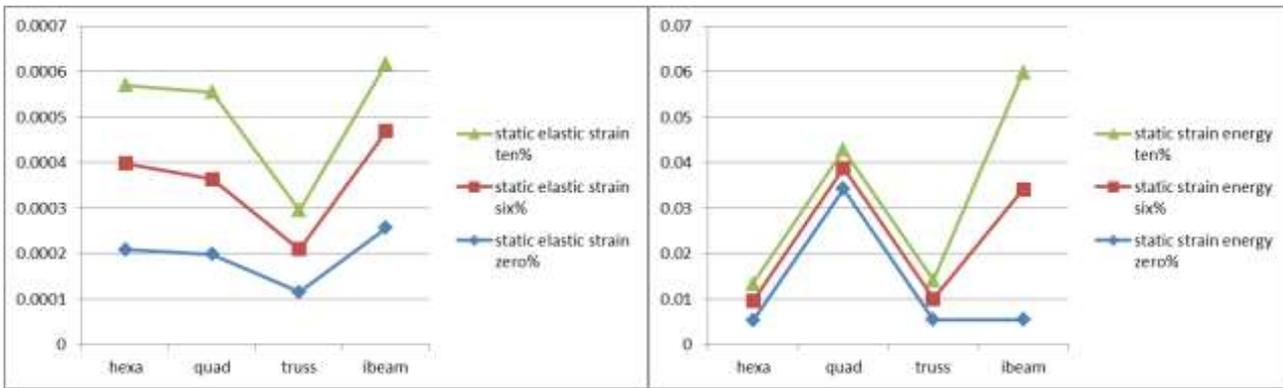
Graph 5.3 Overall elastic strain Graph 5.3 Overall strain energy
