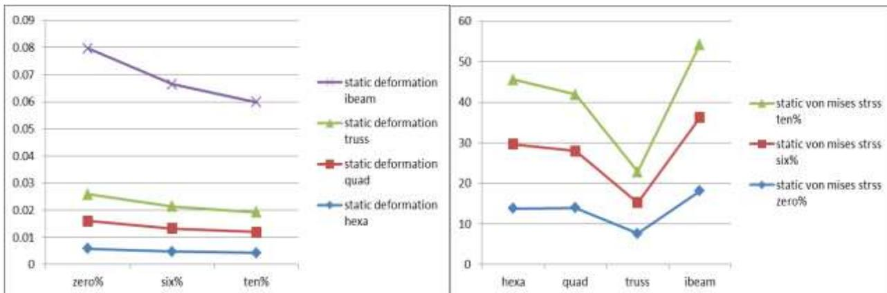
Graph 5.1 Overall static deformation Graph 5.2 Overall vonmises stress
